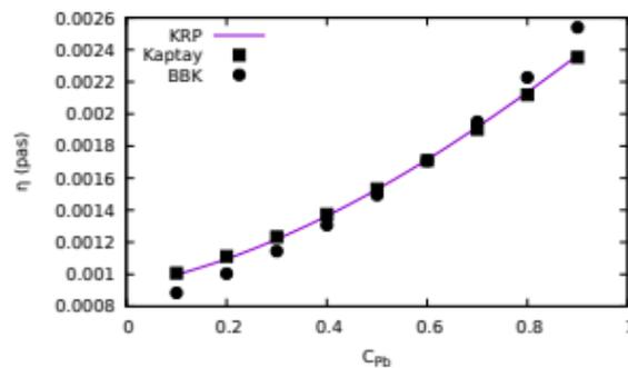
Figure 6: Viscosity versus bulk concentration of Pb
