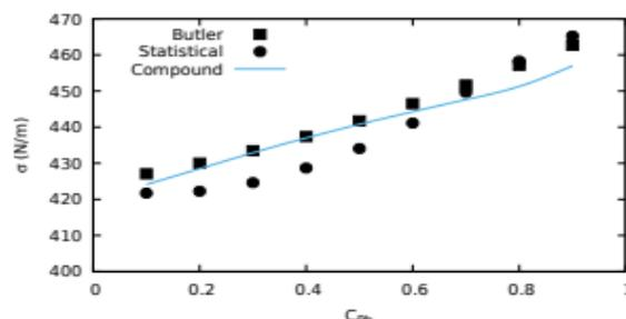
Figure 8: Surface tension versus bulk Pb concentration
