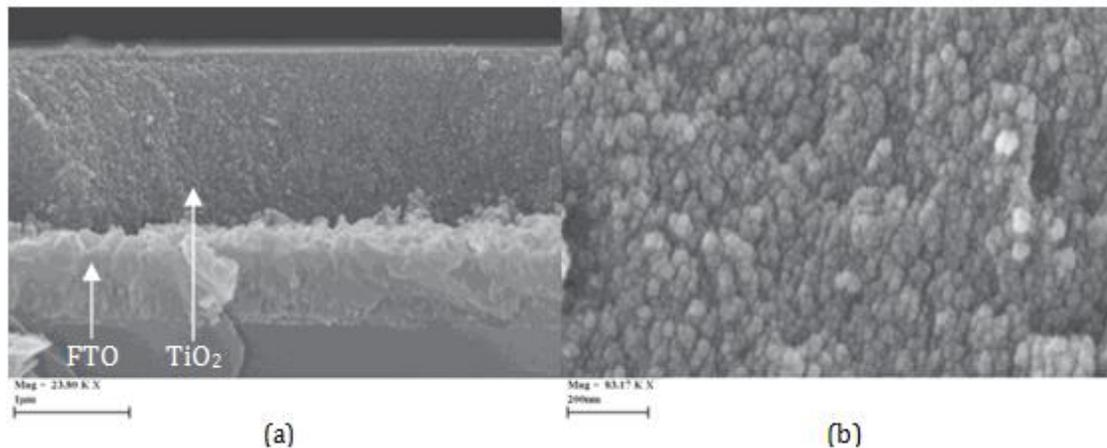
**Fig. 4. TiO<sub>2</sub> nanocrystalline film made of sol-gel procedure (a) cross sectional image and (b) higher magnification of the film.**
