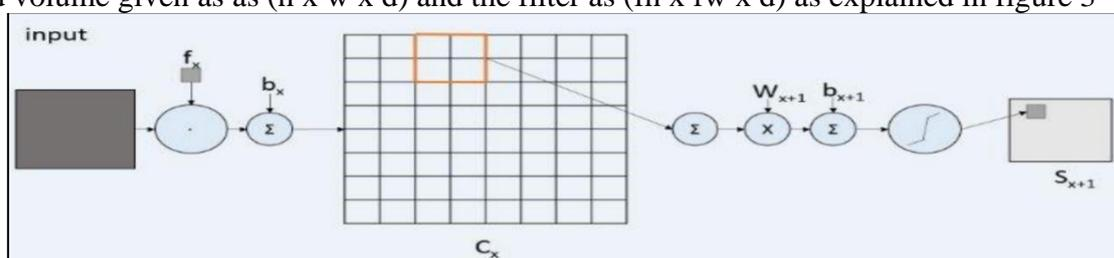
**Figure 3:** Process of Convolution Neural Network (CNN)
