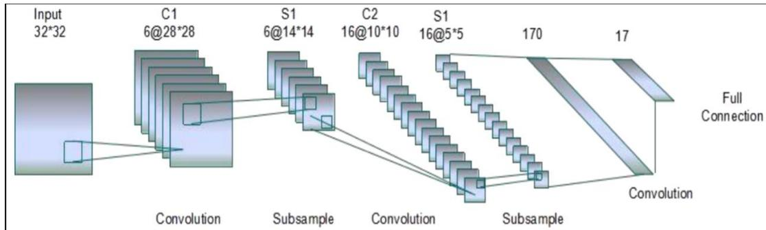
**Figure 4:** Stages of Convolution Neural Network (CNN) model
