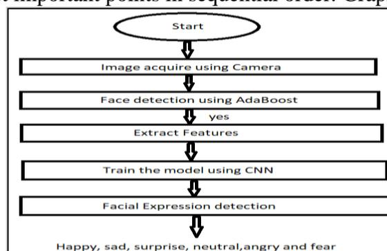
**Figure 12:** Face detection and emotion recognition flow chart
