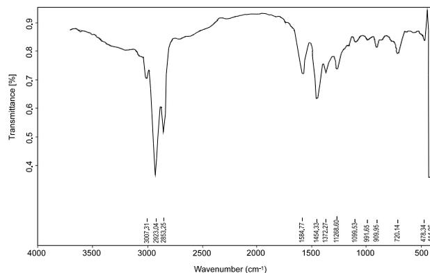
Fig. 3: FT-IR spectrum of CNSL resin-bitumen blend
