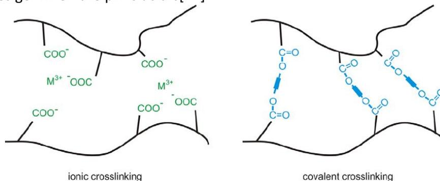
Figure No. 10 Ionic cross-linking(44)
