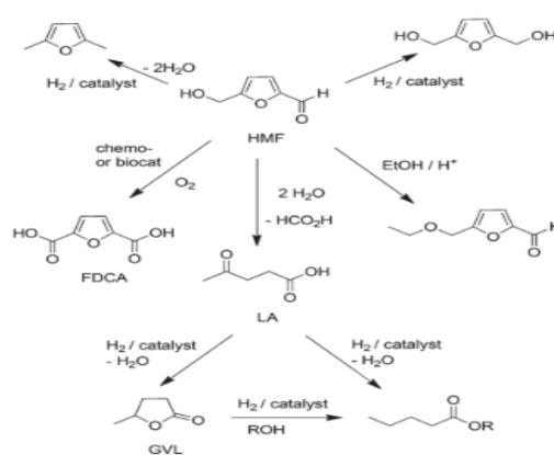
**Figure 3: Catalytic hydroxymethyl furfural conversions to products.**
