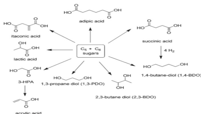
**Figure 1: Biomass-derived sugar fermentation produces commodity chemicals.**
