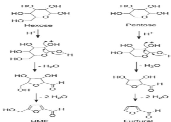
**Figure 2: Using xylose and fructose to make furfural and hydroxymethyl furfural.**
