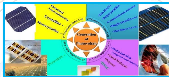
Figure 1 Generation of Photovoltaic solar cells with various materials blend and technology
